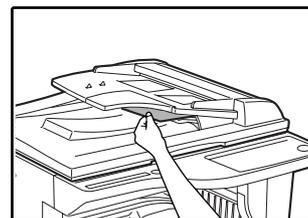
If a small original (5-1/2" x 8-1/2", etc.) is misfed, or if an original misfeed occurs in the reversing tray of the RSPF (if installed), open the right side cover and remove the original. Close the right side cover.
