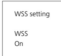
Some TV broadcasters transmit a picture format identification, enabling the TV to switch to the proper format automatically when WSS is On. When WSS is On, detection is carried out on all picture sources, i.e.
