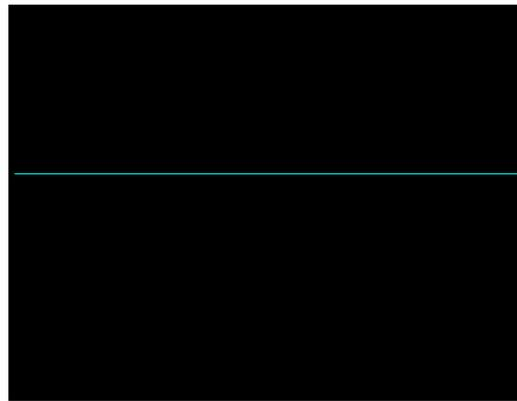
From the option list change option 2 bit 6 from 0 to 1 for disabling vertical scan. Adjust horizontal line via screen adjust pot. as thin as possible. Then press 0 to leave service menu.
