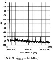
$f_{OUT} = 2.4 \text{ kHz}, \text{ Frequency}$ Word = 000FBA9
