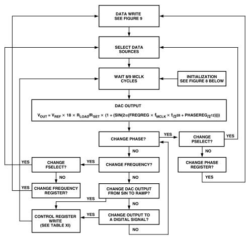
Figure 7. Flow Chart for AD9833 Initialization and Operation
