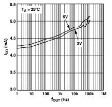
TPC 2. Typical  $I_{DD}$  vs.  $f_{OUT}$  for  $f_{MCLK} = 25 \text{ MHz}$
