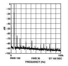
TPC 12.  $f_{MCLK} = 25 \text{ MHz},$  $f_{OUT} = 6 \text{ kHz},$  Frequency Word = 000FBA9
