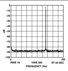
TPC 11.  $f_{MCLK} = 10 \text{ MHz},$  $f_{OUT} = 3.33 \text{ MHz} = f_{MCLK}/3,$ Frequency Word = 5555555
