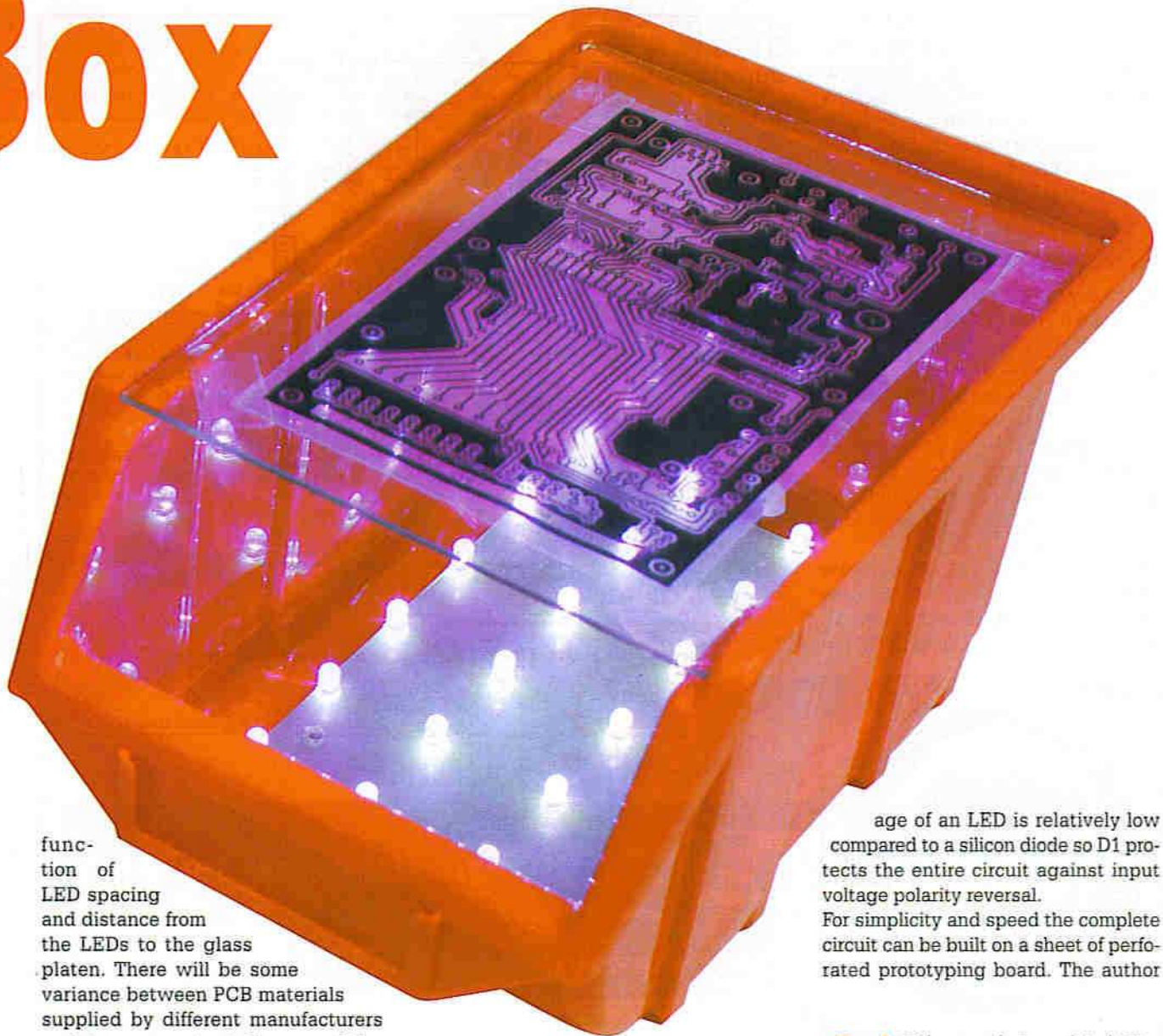
Figure 2. LED layout on the Eurocard sized PCB.
