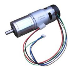
The EMG49 (encoder, motor, gearbox 49:1) is a 24v motor fully equipped with encoders and a 49:1 reduction gearbox. It is ideal for medium to large robotic applications, providing cost effective drive and feedback for the user. It also includes a standard noise suppression capacitor across the motor windings.
