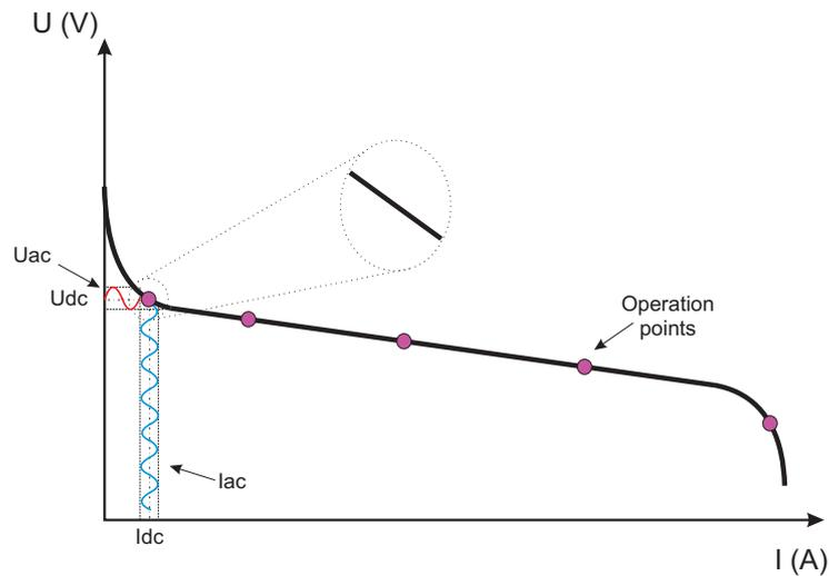
Fig. 4.5: EIS test linearity vs. final model nonlinearity
