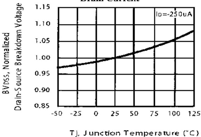
**Fig 5. Breakdown Voltage v.s. Junction Temperature**
