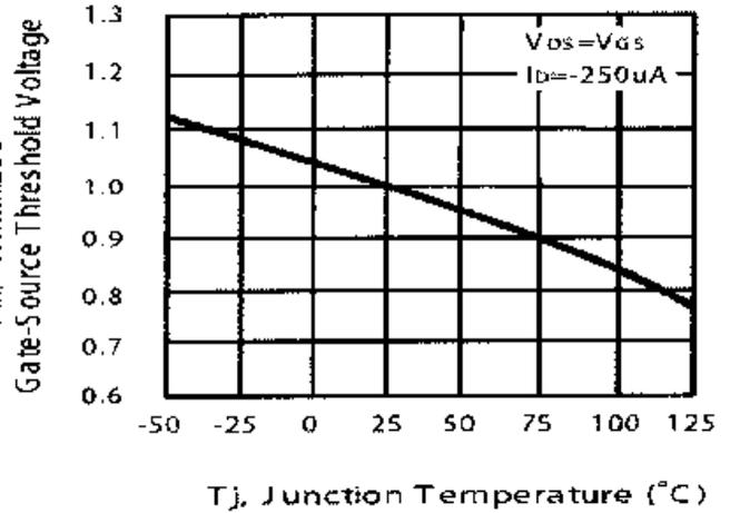
**Fig 8. Gate Threshold Voltage v.s. Junction Temperature**
