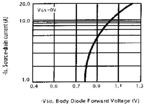
**Fig 6. Body Diode Forward Voltage v.s. Source Current**
