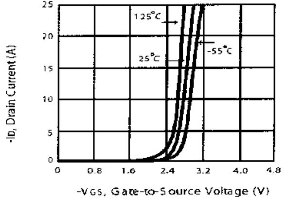
**Fig 2. Transfer Characteristics**
