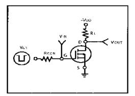
Fig 11. Switching Time Circuit
