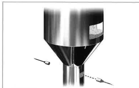
Detecting the level of contents in a hopper.
