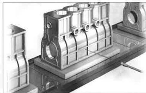
Checking the seating of workpieces for an NC processor.
