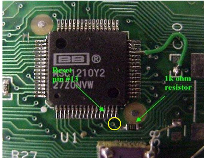
The goal was to place the resistor to protect the reset pin. The close placement of the resistor didn't solve the problem. However the feedthrough was to an external connector that defeated the purpose of the resistor.
