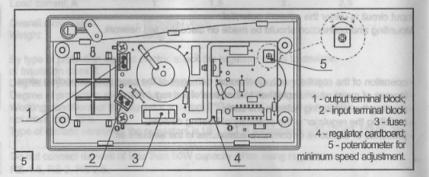
It is necessary to install minimum fan speed with the potentiometer 5 (fig.5), when the fan speed knob 1 (fig.4) is set to the minimum position.
