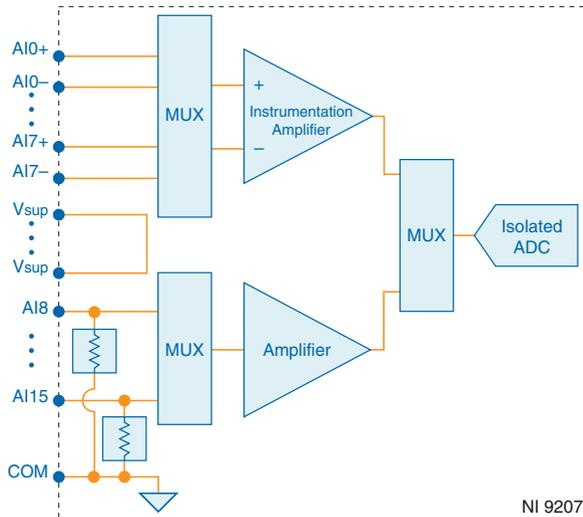
The input signals are scanned, amplified, conditioned, and then sampled by a single 24-bit ADC.
