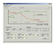
The control software of the Hybrid Extension Kit visualizes all data related to hybridization and battery management. It also allows the user to set different battery types and optimize the charging and discharging parameters.
