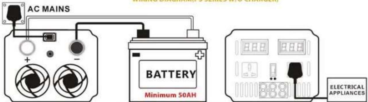
WIRING DIAGRAM(EPS/PS-C SERIES WITH CHARGER)
