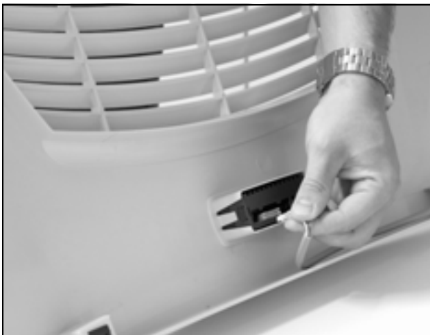
Fig. 24: Disconnect the connector from the display
