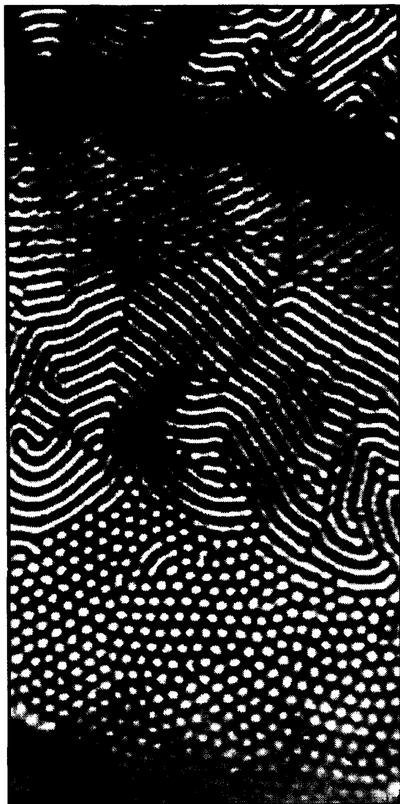
Fig. 6. Transient pattern sequence in the bevelled disc. Note that, as in Fig. 5, the pattern has disappeared over large extents; see the region of homogeneous state located in the upper parts of the figure; see also the black hexagons at the borders of this region. Picture taken 2 h after 10% increase in the chlorite concentration. All other experimental conditions as in Fig. 3.
