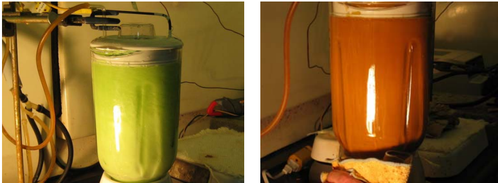
Figure 4 - Blender demonstration test: starting solution and final slurry (10 minutes)
