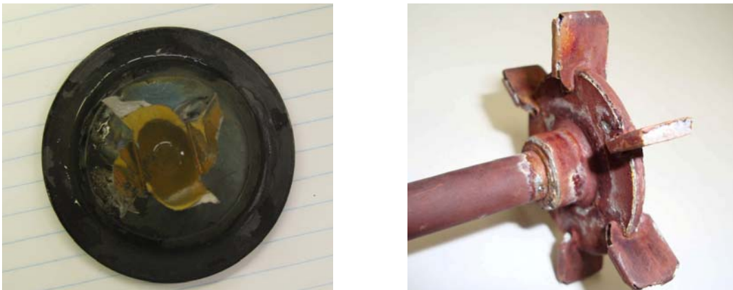
Figure 5 – Impellers at end of oxidation tests (blender, left and coated titanium, right)
