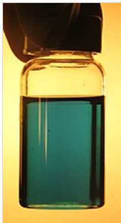
The deep colour of lithium naphthalenide results from the lithium naphthalenide radical .
