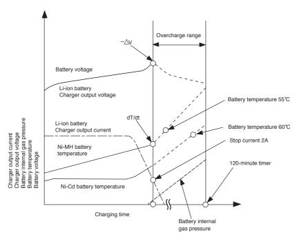
Fig. 7 Relationships of time, voltage, temperature and gas pressure while charging
