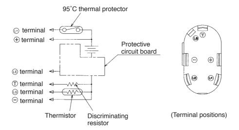
Fig. 6 Li-ion batteries (14.4 V, 18 V)
