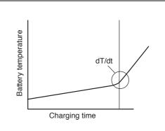
Sudden temperature rise just before full charging is detected and charging is suspended (Ni-MH and SUPER Ni-MH batteries)
