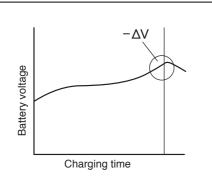
The descending voltage (  $-\,\Delta\,V$  ) of the battery in the final stage of charging is detected, and charging is automatically suspended.
