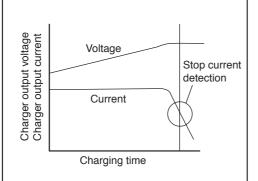
The Model UC 18YRL/UC 18YFL automatically stops recharging upon detection of the stop current only when recharging a lithium-ion battery.
