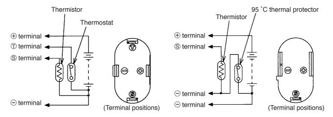
Fig. 2 Ni-Cd batteries (7.2 to 12 V)
