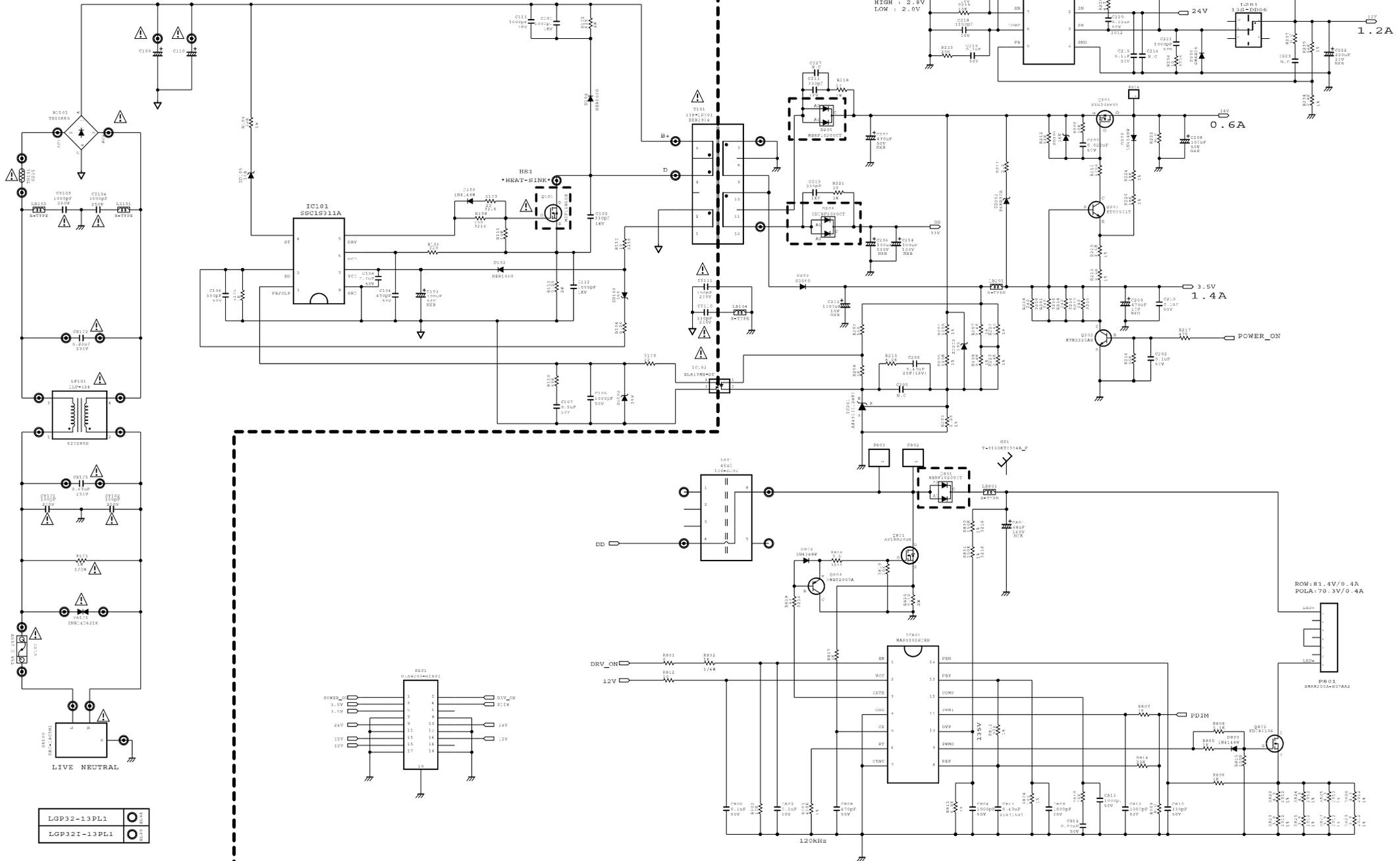
THE  $\Delta$  SYMBOL MARK OF THIS SCHEMATIC DIAGRAM INCORPORATES SPECIAL FEATURES IMPORTANT FOR PROTECTION FROM X-RADIATION. FUSE AND ELECTRICAL SHOCK HAZARDS, WHEN SERVICING IF IS ESSENTIAL THAT ONLY MANUFACTURES SPECIFIED PARTS BE USED FOR THE CRITICAL COMPONENTS IN THE  $\Delta$  SYMBOL MARK OF THE SCHEMATIC.
