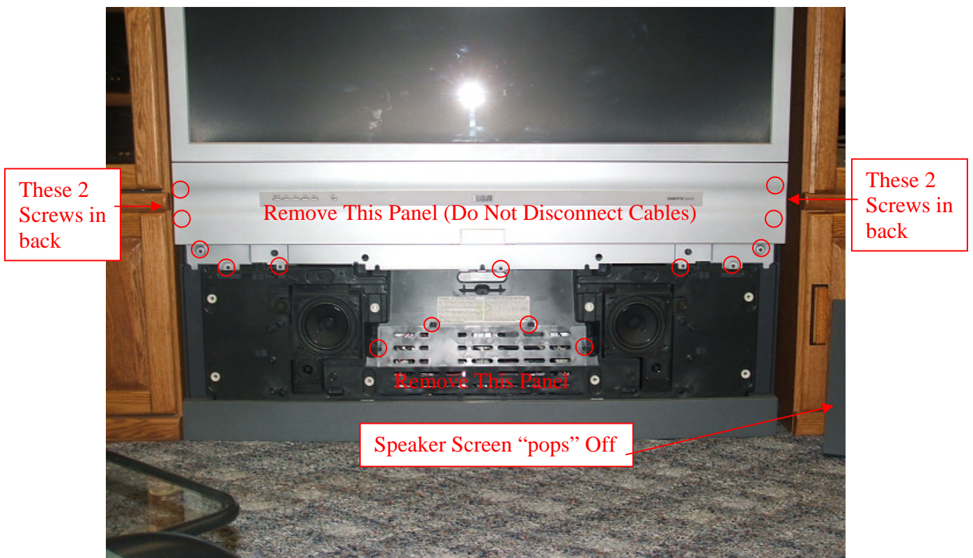
Figure 1: D56W20 with speaker screen removed. Remove the circled screws to release the two panels. Do not disconnect the cables to the power/channel/volume panel
