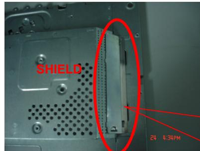
Remove the screws to remove the bezel
