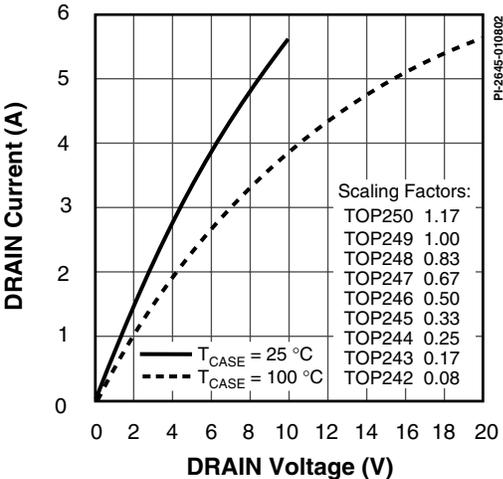
Figure 67. Output Characteristics.
