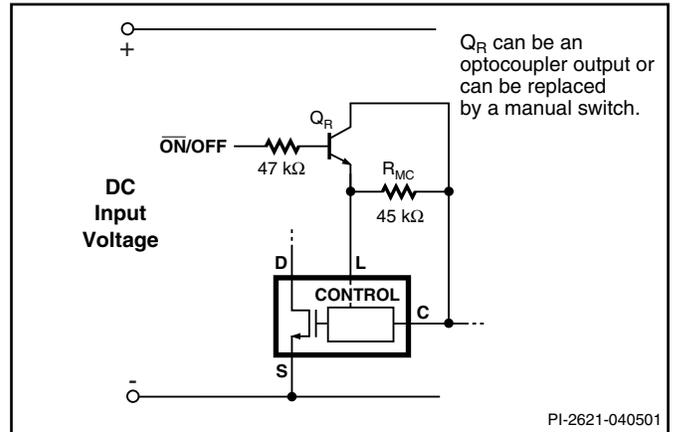
Figure 23. Active-off Remote ON/OFF. Maximum Duty Cycle Reduced.
