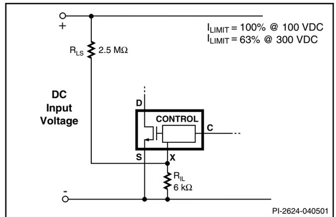
Figure 21. Current Limit Reduction with Line Voltage.
