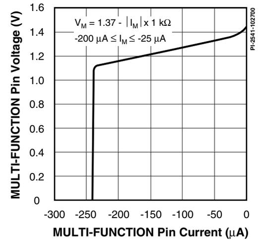
Figure 64b. MULTI-FUNCTION Pin Voltage vs. Current (Expanded).
