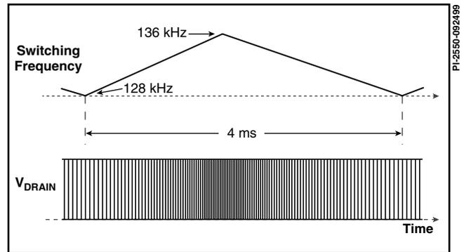
Figure 9. Switching Frequency Jitter (Idealized  $V_{DRAIN}$  Waveforms).
