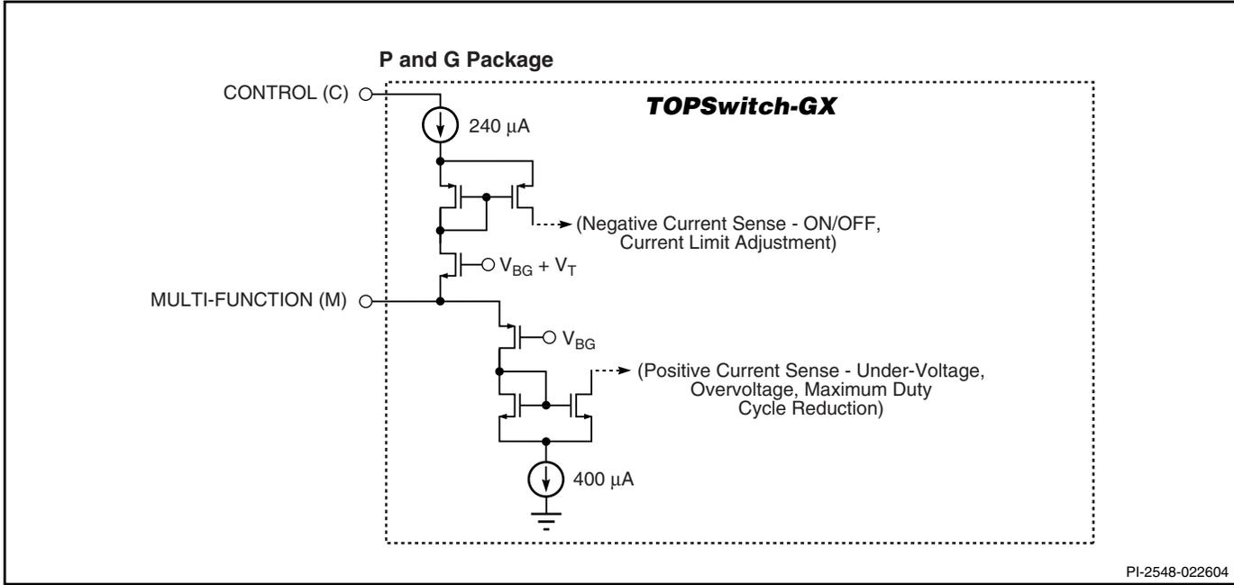
Figure 12b. MULTI-FUNCTION (M) Pin Input Simplified Schematic.
