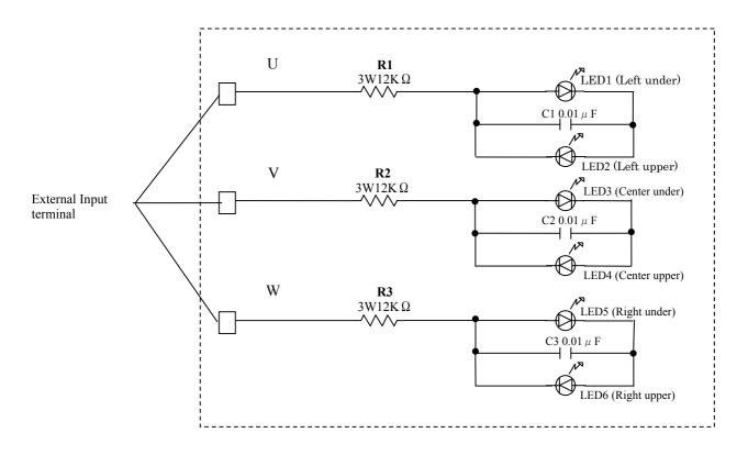
Fig.3 Internal Circuit of the Inverter Analyzer
