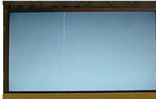
Vertical Line Source TAB IC Defect
