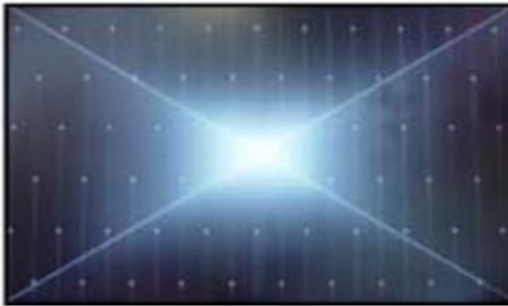
Solder defect, Short/Crack
