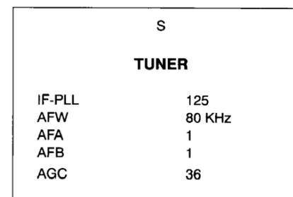
When the main signal processor (IC TDA8374/75) is changed, the IF PLL needs to be realigned as follows:
