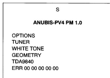
General: The items of the sub menus in the Service Menu can be selected with the up/down arrow keys on the remote control. Entry into the sub menus is executed with the east/west arrow keys. Leaf the sub menu via the "OK" key. In the Service Menu the following information and sub menu items are indicated.
