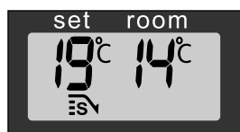
I: When the SAVE function is activated, the heater will automatically switch on or off in order to remain within a specified temperature range.
