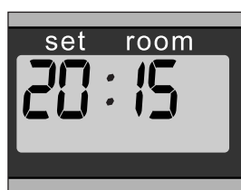
E: When the 4-digit stops blinking, the setting has been locked to the indicated value.
