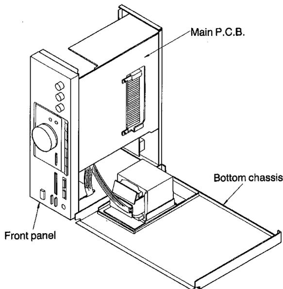
5. Remove the bottom chassis.
