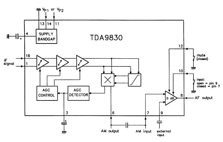
combination with the frequency response of the IF amplifier applications in a frequency range from approximately 6 MHz up to 70 MHz are possible.
