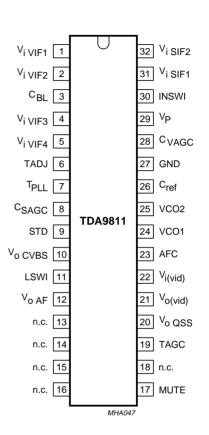
Fig.2 Pin configuration.
