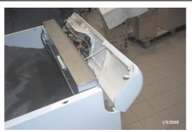
Fig. 6 - Turn the control panel forwards.
