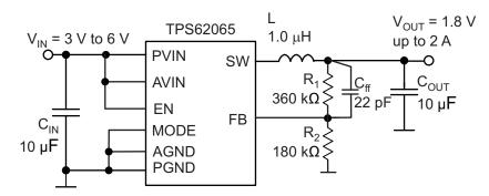
Figure 26. TPS62065 1.8V Adjustable Output Voltage Configuration
