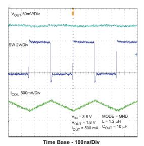
Figure 13. Typical Operation (PWM Mode)
