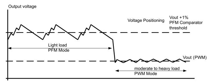
Figure 24. Power Save Mode Operation with automatic Mode transition
