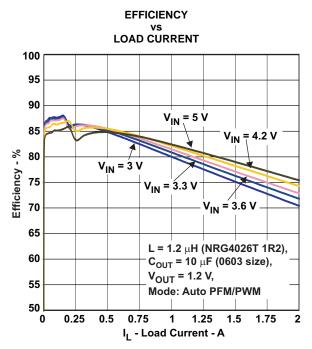
Figure 1. V<sub>OUT</sub> = 1.2V, Auto PFM/PWM Mode, Linear Scale
