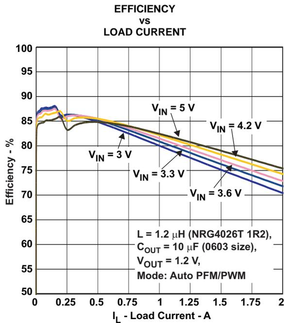
Figure 1.  $V_{OUT} = 1.2V$ , Auto PFM/PWM Mode, Linear Scale
