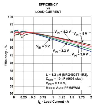
Figure 2. V<sub>OUT</sub> = 1.8V, Auto PFM/PWM Mode, Linear Scale
