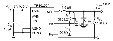
Figure 27. TPS62267 Adjustable 1.8-V Output
