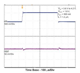
Figure 18. Line Transient Response PWM Mode
