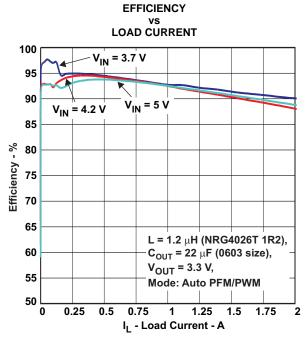
Figure 3. V<sub>OUT</sub> = 3.3V, Auto PFM/PWM Mode, Linear Scale
