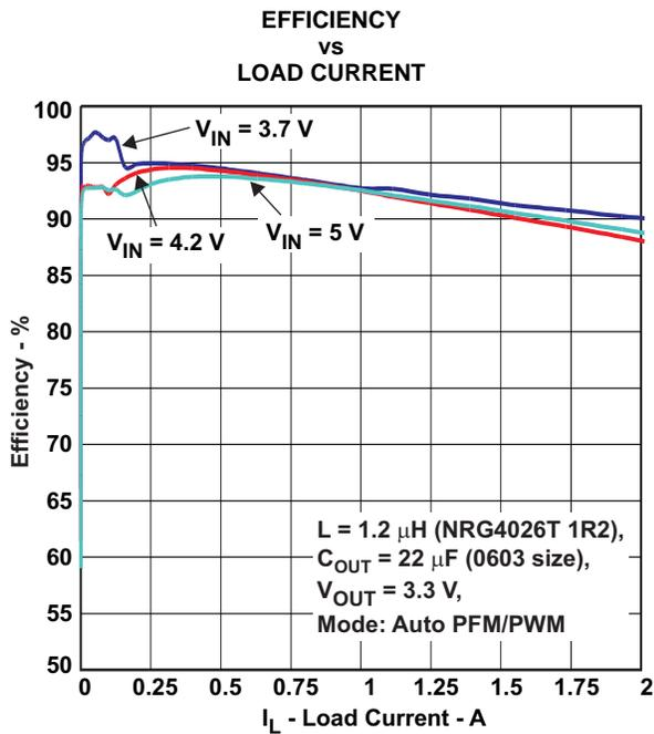
Figure 3.  $V_{OUT} = 3.3V$ , Auto PFM/PWM Mode, Linear Scale
