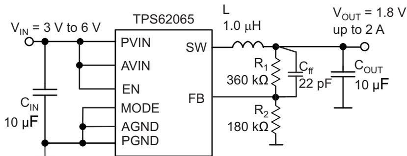
Figure 26. TPS62065 1.8V Adjustable Output Voltage Configuration
