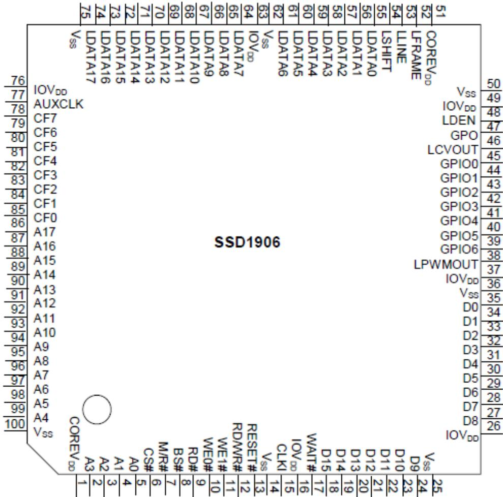
**Figure 4-2 : Pinout Diagram – 100 pin TQFP**
