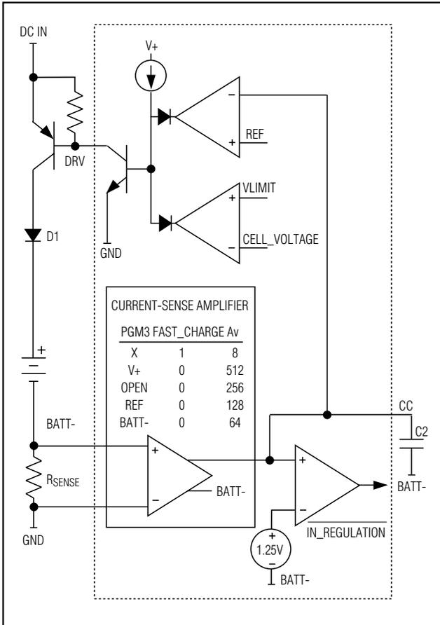
Figure 6. Current and Voltage Regulator (linear mode)
