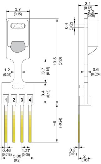
Figure 17 SHT7x dimensions in mm (inch)
