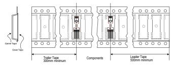
Figure 16 Tape configuration and unit orientation
