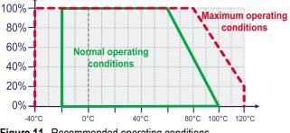
Figure 11 Recommended operating conditions
