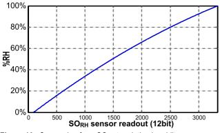
Figure 10 Conversion from SORH to relative humidity
