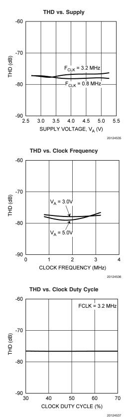
**Typical Performance Characteristics**  $T_A = +25^{\circ}C$ ,  $f_{SAMPLE} = 50$  kSPS to 200 kSPS,  $f_{SCLK} = 0.8$  MHz to 3.2 MHz,  $f_{IN} = 39.9$  kHz unless otherwise stated. (Continued)
