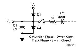
FIGURE 5. Equivalent Input Circuit
