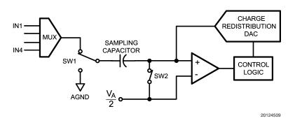
FIGURE 1. ADC084S021 in Track Mode
