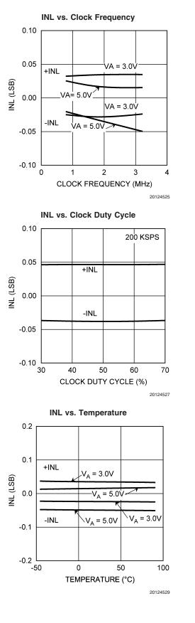
**Typical Performance Characteristics**  $T_A = +25$ °C,  $f_{SAMPLE} = 50$  kSPS to 200 kSPS,  $f_{SCLK} = 0.8$  MHz to 3.2 MHz,  $f_{IN} = 39.9$  kHz unless otherwise stated. (Continued)
