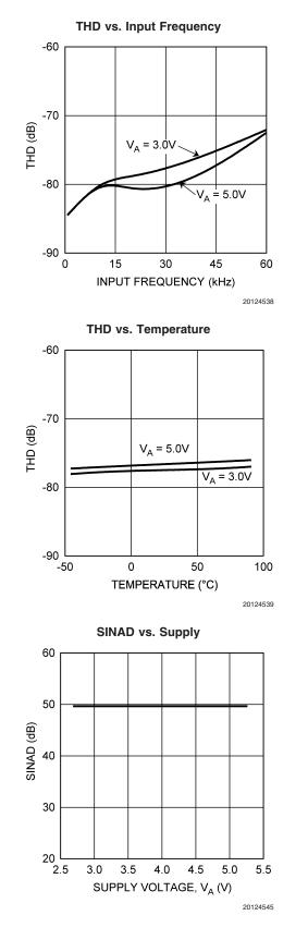
**Typical Performance Characteristics**  $T_A = +25^{\circ}C$ ,  $f_{SAMPLE} = 50$  kSPS to 200 kSPS,  $f_{SCLK} = 0.8$  MHz to 3.2 MHz,  $f_{IN} = 39.9$  kHz unless otherwise stated. (Continued)
