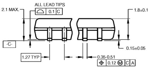
DIMENSIONS ARE IN MILLIMETERS
