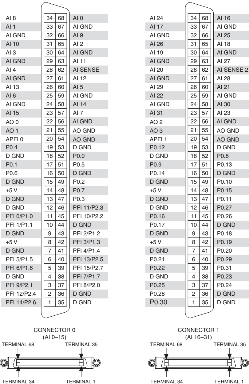
Figure 13. NI USB-6259 Mass Termination Pinout
