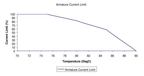
Figure 6: Armature Thermal Cutback Characteristic
