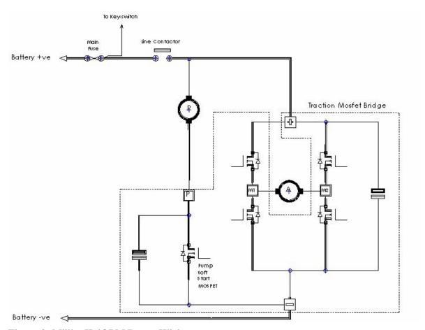
Figure 2: MillipaK 4QPM Power Wiring
