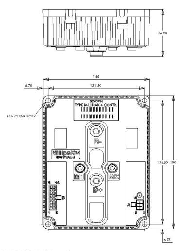
Figure 1: MillipaK 4QPM HP Dimensions
