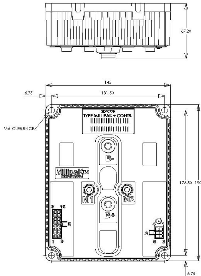
**Figure 1: MillipaK 4QPM HP Dimensions**
