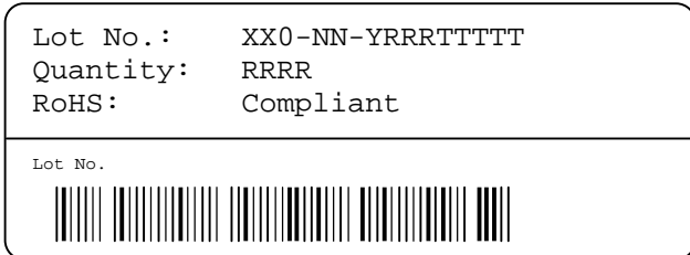
Figure 19: First label on reel: XX = Sensor Type (11 for SHT11), NN = Chip Version (04 for V4), Y = last digit of year, RRR = number of sensors on reel divided by 10 (200 for 2000 units), TTTTT = Traceability Code.
