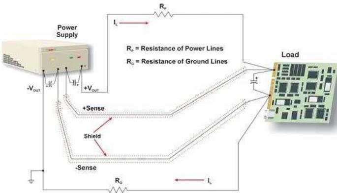
**Figure 7: Remote Sensing**
