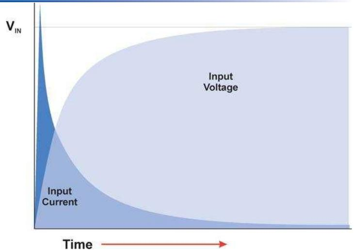
**Figure 9: Input Current vs Input Voltage**
