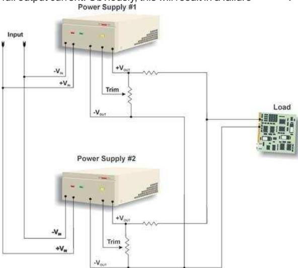
**Figure 17: Parallel Connection, Multiple Units**
