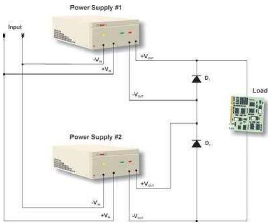
**Figure 16: Series Connection, Multiple Units**
