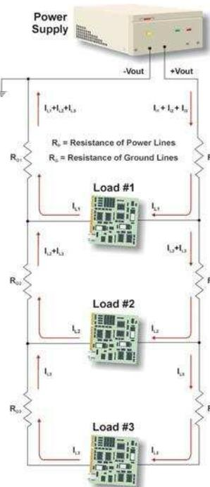
Figure 2: Parallel Power Distribution
