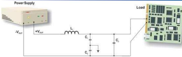
Figure 13: Output Filtering
