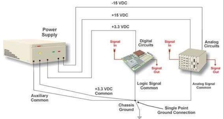
Figure 5: Analog-Digital Connection
