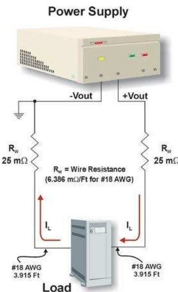
Figure 1: Power Line Resistance
