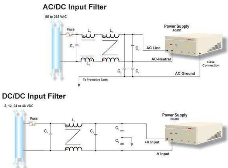
Figure 12: Input Filtering
