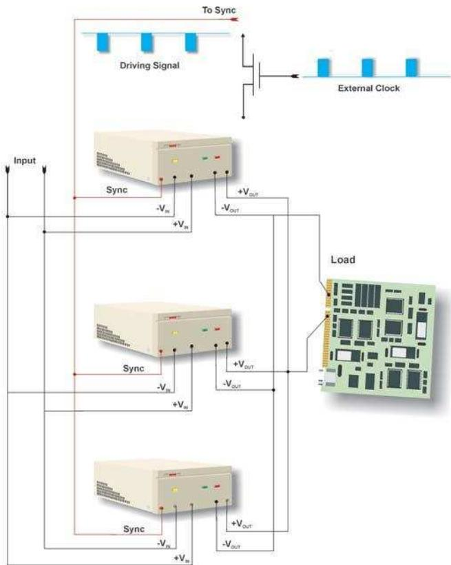
Figure 11: External Clock Connection
