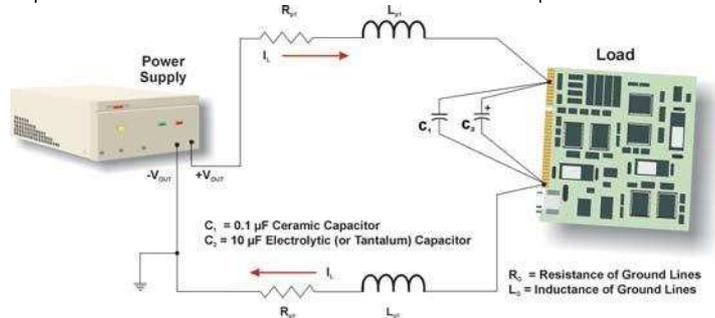
Figure 6: Load Decoupling
