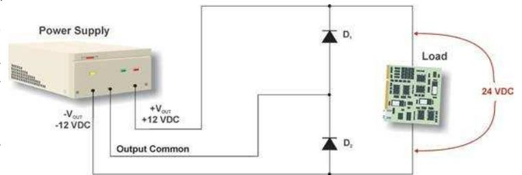
Figure 15: Output Series Connection
