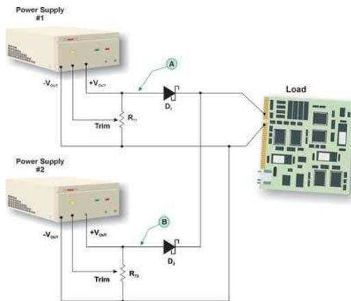
**Figure 18: Dual Redundant Connection**
