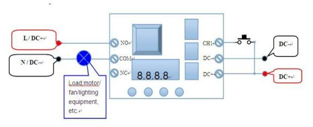
Gentle remind: If user load and FRM01 module use a seam DC power supply, it is possible because of the power supply capacity is insufficient or wiring connections unfit, the module appears unstable phenomenon occasionally, please use the following (even if no found the problem, it should follow the recommendations):
