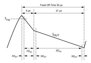
Figure 2. Mixed Decay Mode Operation
