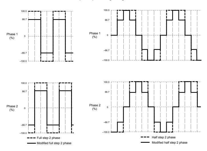
Figure 3. Step Sequencing for Full-Step Increments.
