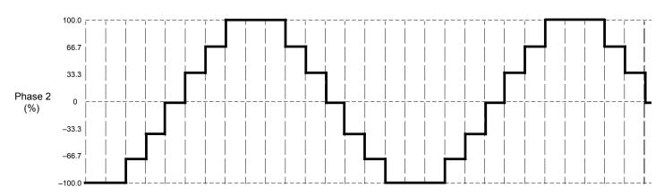
Figure 5. Decay Modes for Quarter-Step Increments
