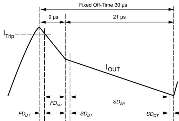
Figure 2. Mixed Decay Mode Operation
