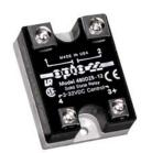
Opto 22 provides a full range of Power Series relays with a wide variety of voltage (120–575 volts) and current options (3–45 amps). All Power Series relays feature 4,000 volts of optical isolation and have a high PRV rating. Some Power Series relays include built-in LEDs to indicate operation. See page 4.
