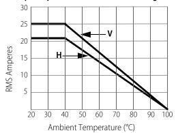
V. Heatsink mounted to a vertical surface **H**: Heatsink mounted to a **horizontal** surface.
