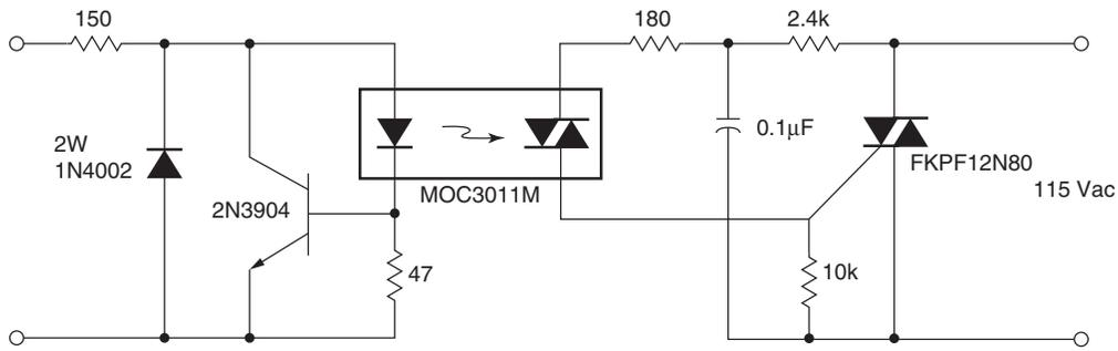
Figure 9. Solid-State Relay
