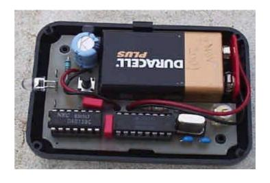
The trimmer (C1) can be omitted and both load capacitors (C2, C3) for the crystal made equal (around 27pF, although the value is not critical. Anthing from 15p to 47p should work. At low battery voltages (5v), oscillation is less reliable and may be less tolerant of non-optimal capacitor values.
