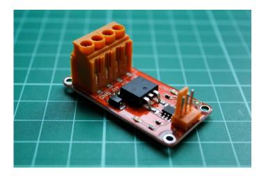
This module switches a high current load using a high power transistor. Unlike a mechanical relay, this is capable of high speed switching for use with PWM.
