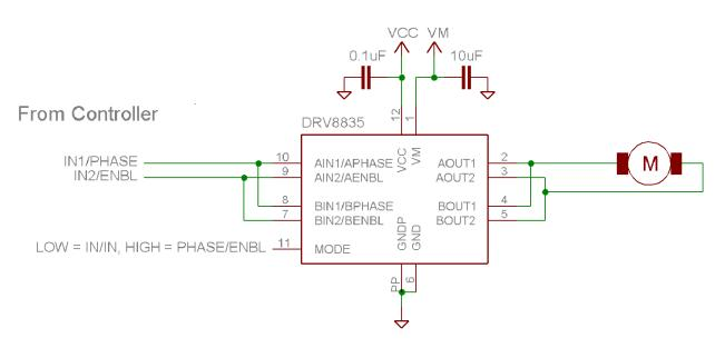
Figure 1. Parallel Mode Connections
