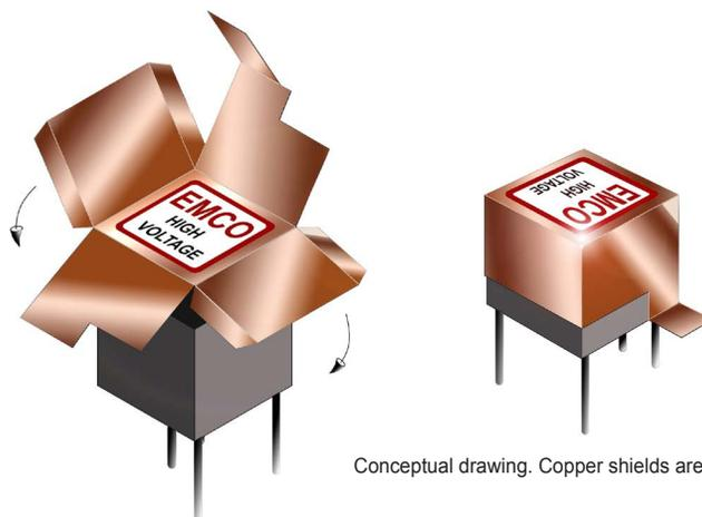
Conceptual drawing. Copper shields are factory installed.
