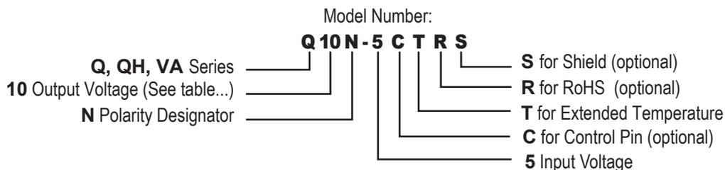
EXAMPLE - **Q10N-5CTRS**: **Q** Series 0.5W, **1000** VDC, **N** negative, **5** VDC input, **C** for Control Pin, **T** for Extended Temperature, **R** with RoHS, **S** for Shield.
