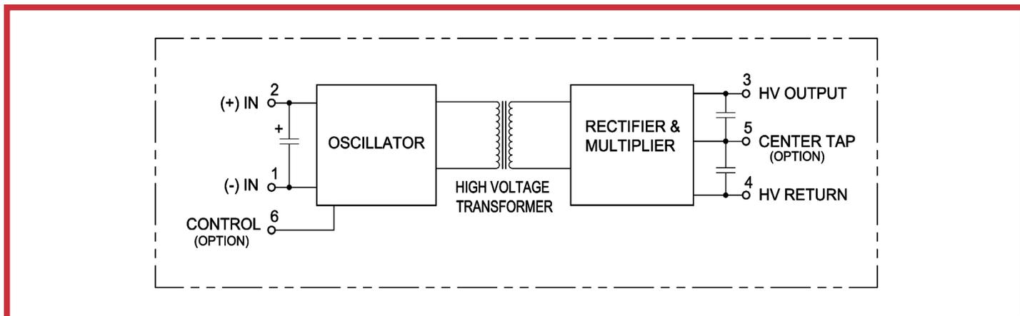
NOTE: Pin designators for pin out models up to 5KV.
