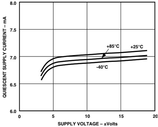
Figure 5. Quiescent Supply Current vs. Supply Voltage
