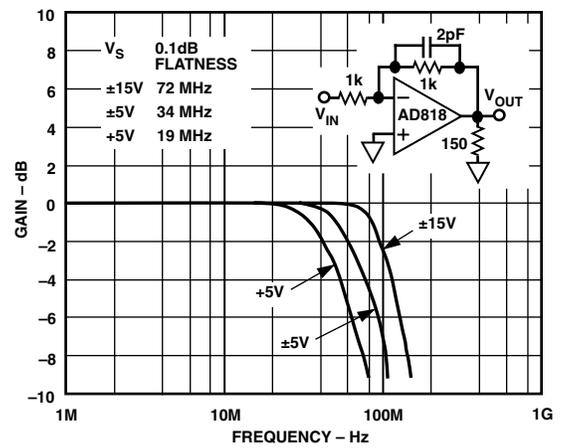
Figure 21. Closed-Loop Gain vs. Frequency ( $G = -1$ )
