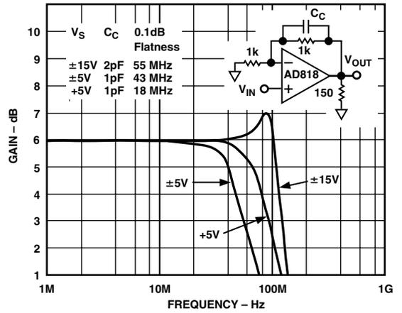
Figure 20. Closed-Loop Gain vs. Frequency ( $G = +2$ )
