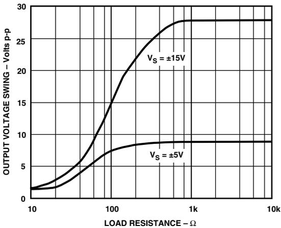
Figure 2. Output Voltage Swing vs. Load Resistance
