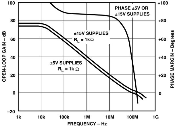
Figure 11. Open-Loop Gain and Phase Margin vs. Frequency
