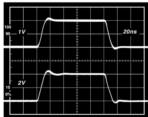
Figure 40. Performance of Line Receiver,  $R_L = 150 \Omega$ ,  $G = +2$
