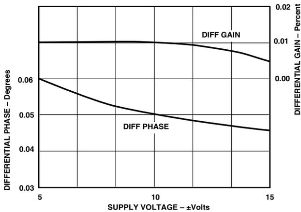
Figure 19. Differential Gain and Phase vs. Supply Voltage
