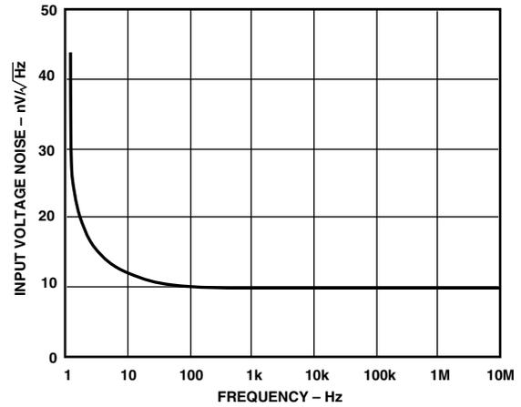
Figure 15. Input Voltage Noise Spectral Density vs. Frequency
