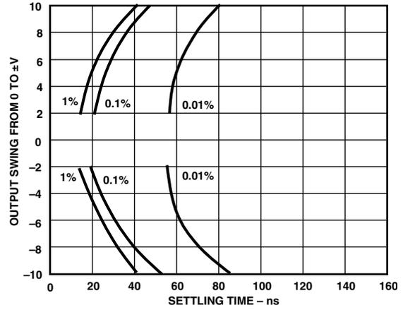
Figure 14. Output Swing and Error vs. Settling Time
