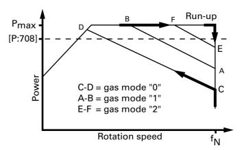
Fig. 6: Principle of power characteristics lines for gas type dependent operations, e.g. gas mode = 0
