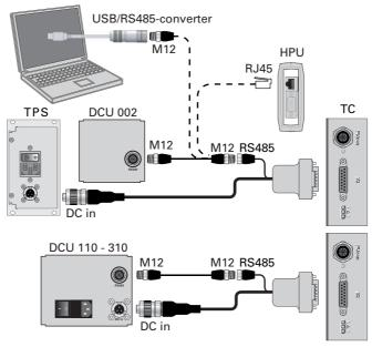
Fig. 4: Optional connection possibilities for interface RS485
